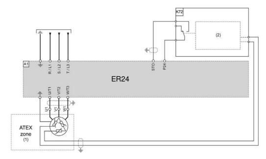
ATEX Zone 1/21 or 2/22 with at least 1 thermal sensor PTC type ATEX certified control unit conversion / insulation / switching system with Level of protection intrinsic safety"i". (K72) ATEX certified PTC relay
